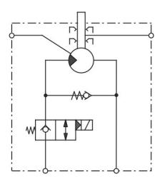
QXM internal gear motors with make-up valve, ON/OFF valve, external drain port, sealing variant for ultra-high protection against external leakage, and tell-tale hole.
