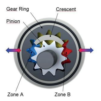
The special design is crucial in ensuring that the QXM internal gear motor starts up optimally, operates quietly and delivers stable torques, even at high speeds. These advantages are based on the long pressure-decay zone around the crescent and the special features of the gear profile.
