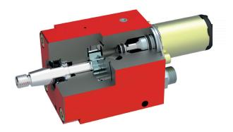
On request, users can get the QXM internal gear motors with integral valve functions. Bucher Hydraulics offers the direct mounting of pressure relief, make-up and flow control valves. In addition, directional control valves enable the unit to be switched on and off and changed from left- to right-hand rotation.
